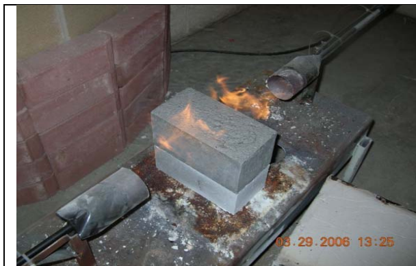
Figure 4: Heat being applied to two sides of a cured Thermbond material
