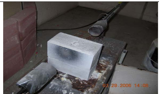
Figure 5: After 50 minutes of firing; no cracking or spalling of sample
