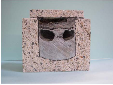
Fig. 1: Aleris /TATA cup test at 900°C
