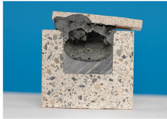
Figure 6. Castable refractory cup test shows phosphate-bonded materials are resistant to high Mg-alloys.
