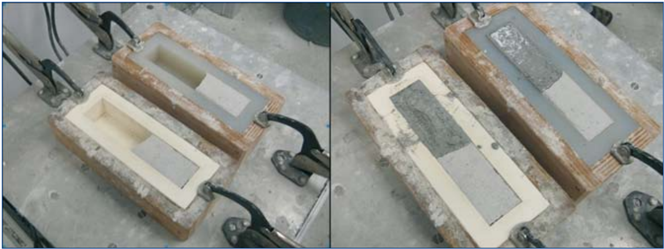
Figure 3. Preparation of composite samples for bond strength test.
